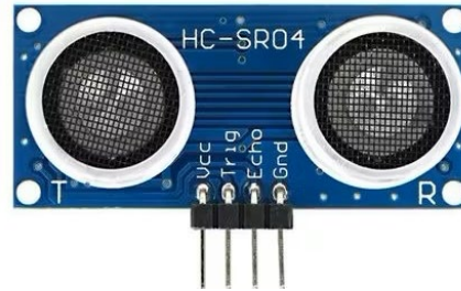
Figure 4: pin layout for the ultrasound sensor; VCC is for a 5V supply, Trig starts an ultrasound echo pulse when activated, Echo tells when the echo pulse has returned to the sensor, and GND is standard ground.
